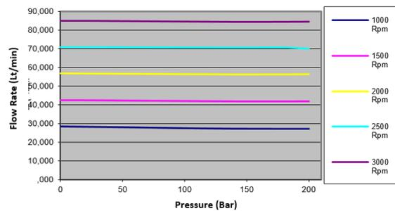
**Fig. 16** Flow rate variation with pressure for increasing speed (Fifth gear pump)
