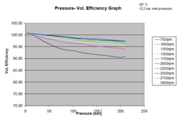
**Fig. 4.** Volume efficiency of gear pumps with pressure for different rpm values
