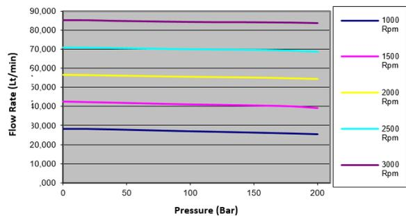
**Fig. 10** Flow rate variation with pressure for increasing speed (Second gear pump)
