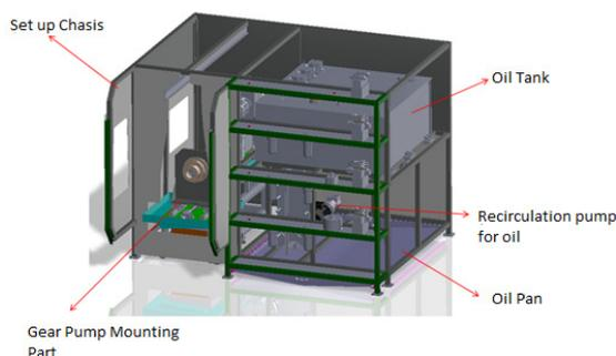
**Fig. 1.** Gear pump test setup chassis
