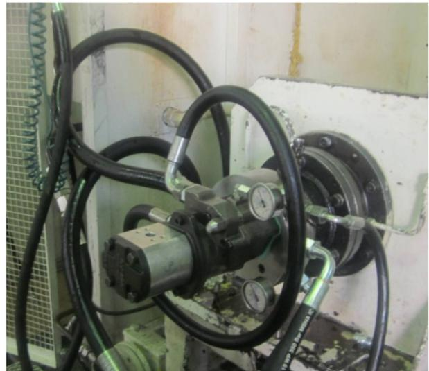
**Fig. 5.** Connection of gear pumps to test setup
